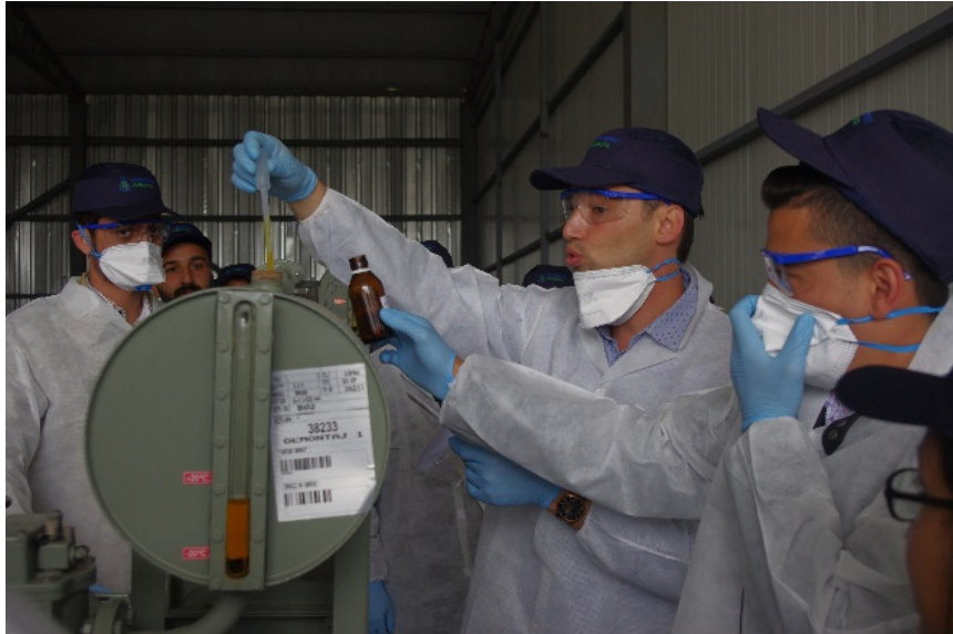
Figure 2.5 Getting Sample from the Top of the Transformer
