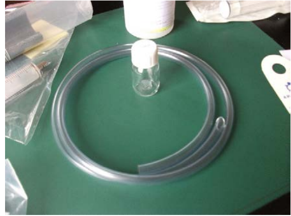
2. Pipe: « CRISTAL 8X1.5 1T/11 » and small glass bottle with a plastic cap
